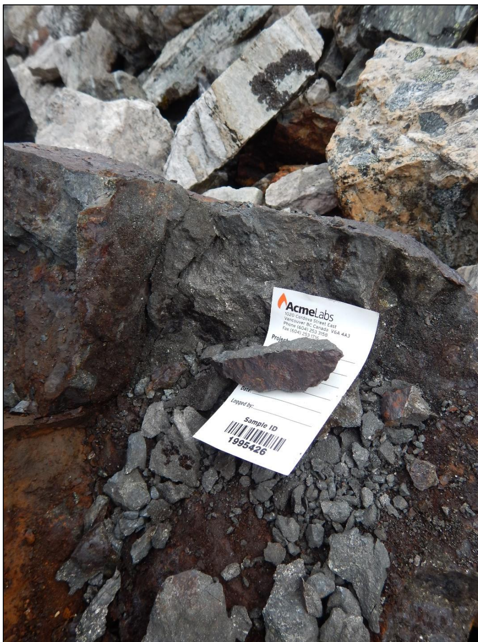
Figure 2: 2020 Discovery: Boulder of massive magnetite-pyrrhotite-chalcopyrite skarn mineralization
